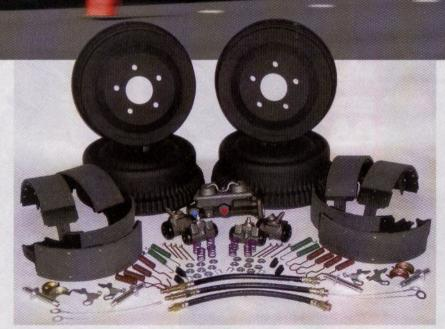
Muscle Car Brakes' drum brake replacement kits for Mopar E-Bodies are available in either 10- or 11-inch configurations. The kits feature cryogenically treated composite brake drums paired with Semi-Ceramic Matrix composition brake shoes, which offer a friction coefficient that's higher than OE. Also included are high-volume wheel cylinders, a high-volume master cylinder and a Heavier Trick Spring Kit.
